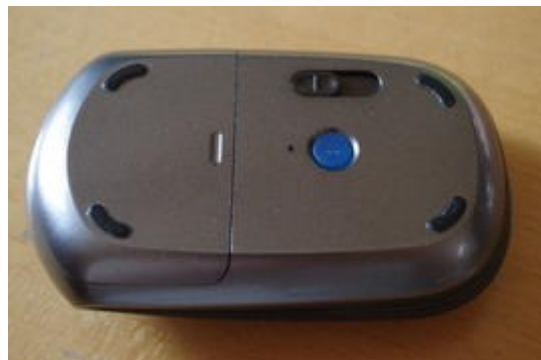
Optical sensor cover and Bluetooth Pairing Button
